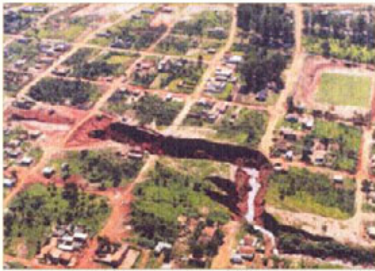
Figure 3.6. Erosion of unprotected urban area (Campana, 2004)
