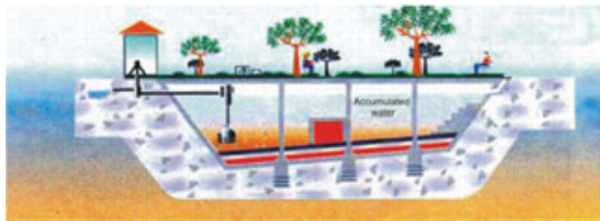
Figure 3.34. Covered detention system (DAEE)
